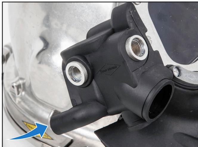
7) Reinstall all of the side block parts that were removed except the bent tube assembly and torque. Refer to “1.3.3 Reassembly of the Defogger Valve” on page SSB-8 and “1.4.3 Reassembly of Emergency Valve (EGS Valve)” on page SSB-13 in the KMDSI modular manual.
