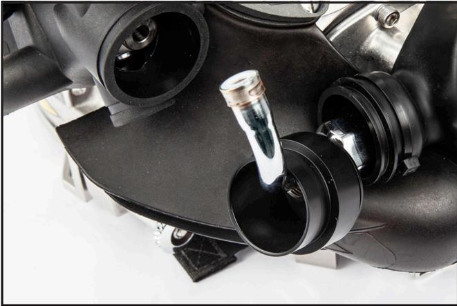
12) Swing the bent tube away from the side block and put the adapter sleeve (short), P/N 550-572, onto the bent tube assembly first, channeled end facing away from regulator inlet.
