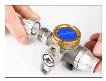
2) Perform vacuum tests for 10 seconds.
