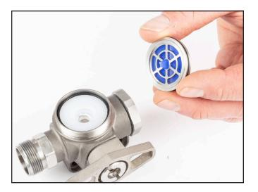
2) Remove O-ring from valve seat.
