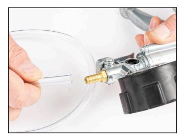
2) Thread test adapter and secure test fixture to the exhausting side of the SBV.
