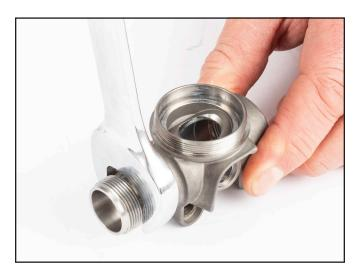
9) Remove sealing O-ring from fitting.
