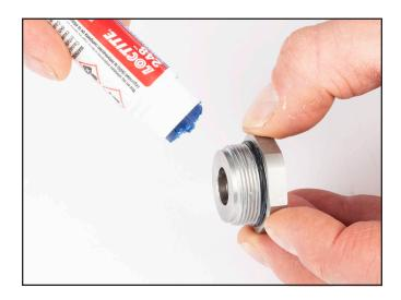
2) Ensure control handle is in the parallel position. Thread adapter on main body. FINAL TORQUE must be applied with SBV secured in a table vise, see "1.3.5 Final Torque" on page KMSBV-14
