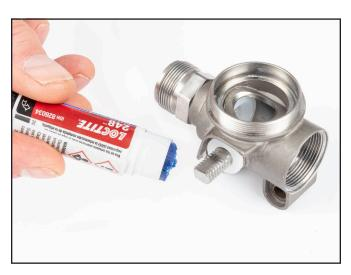
8) Assembly the remainder of the control handle components.
