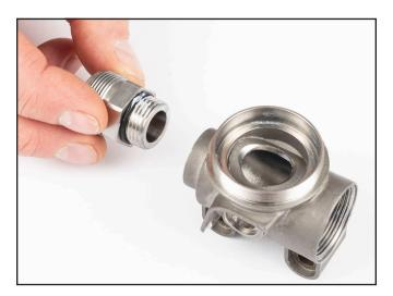
4) Lubricate Ball Seat and outer ball seal surface. The concave end should face toward the center of the SBV body. Seal will fit snug and must be pushed in as far as possible into the body.
