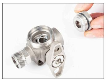
2) Insert tipped end of pick into recessed edge of Ball Seal and remove.
