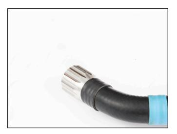
2) Attach the hose assembly to the surface bypass valve assembly (locate blue indicator on hose as show).
