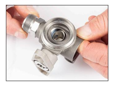
13) Lubricate and insert Ball Seat with concave edge facing into the body. The flat surface of the Ball Seat faces towards the hose fitting adapter.
