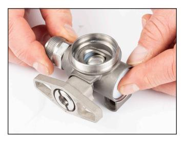
Verify correct orientation – Parallel - OPEN to the exhaust hose. Bypass port will be CLOSED.
