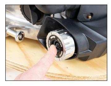
When bubbles appear that is the indication the water dump valve is opening.
