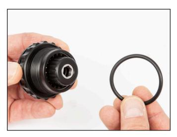
2) Use pick to remove Retaining Ring.
