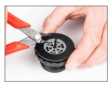
7) Lightly lubricate Compression Sleeve and insert into main body.
