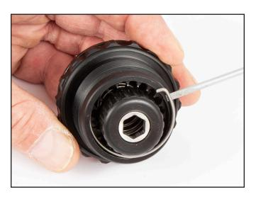
3) Remove the Retaining Cap.
