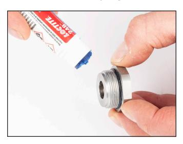
2) Ensure control handle is in the parallel position. Thread adapter on main body. FINAL TORQUE must be applied with SBV secured in a table vise, see "1.3.5 Final Torque" on page KMSBV-14
