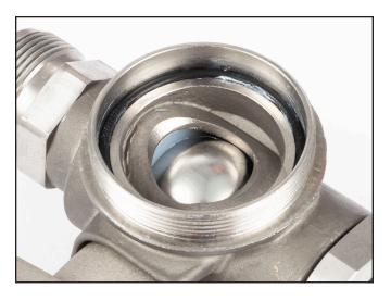
2) Lubricate exposed ball surface and cycle valve handle serval times.
