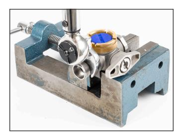
2) Torque Hose Fitting Adapter to final torque.
