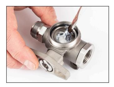
3) Push the Exhaust Port Seal **FIRMLY DOWN** into the body.
