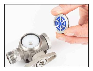
2) Remove O-ring from valve seat.
