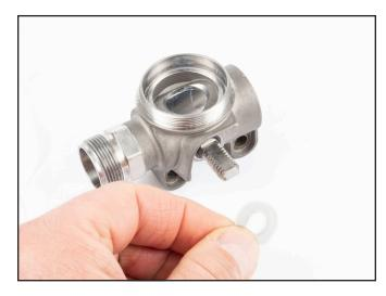
6) Be sure to clean thread locker off of stem threads prior to reassembly.
