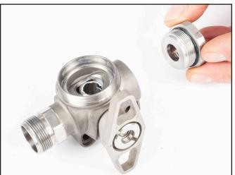
2) Insert tipped end of pick into recessed edge of Ball Seal and remove.
