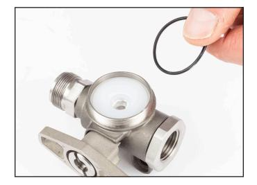
5) Install Butterfly Valve Seat onto correct side of seat.
