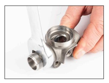
9) Remove sealing O-ring from fitting.
