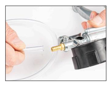
2) Thread test adapter and secure test fixture to the exhausting side of the SBV.
