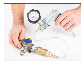
3) Perform Vacuum tests for 10 seconds:
