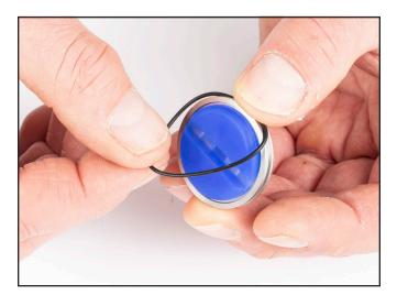
7) Place Butterfly Valve assembly on top of Exhaust Port Seal and O-ring.
