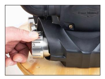
2) Place Water Purge Assembly exit port in a small cup of water.
