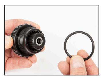
2) Use pick to remove Retaining Ring.
