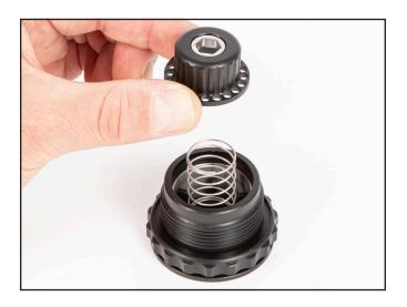
13) Insert Retaining Ring to complete installation.
