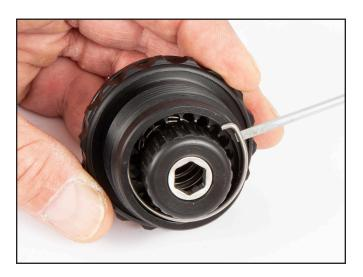
3) Remove the Retaining Cap.
