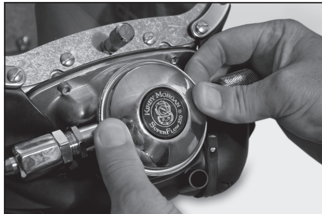
Press the cover over the diaphragm.
