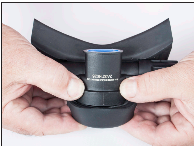
Continue pushing the cover onto the regulator.
