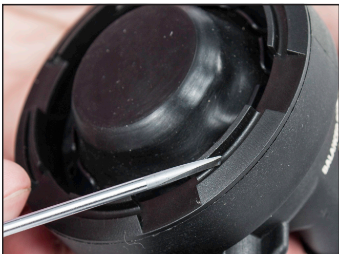
Notice the recessed groove on the diaphragm retaining ring.
