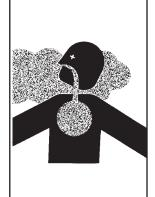
Use silicone sealant in a well ventilated area. Do not breathe the fumes from uncured silicone sealant. These fumes are dangerous and can cause unconsciousness. They can also cause long term damage to body tissue. Read and follow all precautions listed on the silicone sealant tube and Material Safety Data Sheet.
