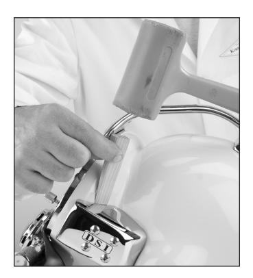
Use a wooden wedge and the mallet to break the seal between the weight and the helmet shell.
