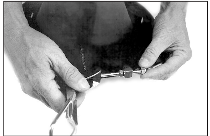
Insert the stud through the block and screw the nut onto the adjustment stud.
