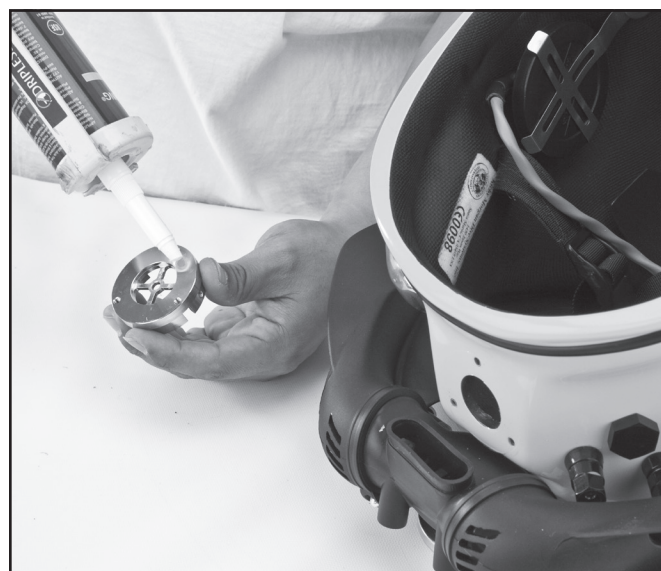
Silicone sealant is used to seal the water dump body to the helmet shell.
