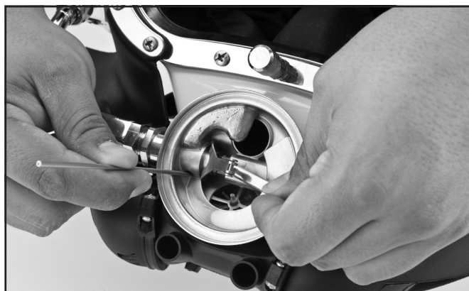
Insert the inlet valve holding tool into the balance hole on the inlet tube.
