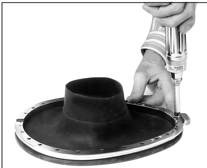
Use the screw to punch through the neck dam.
