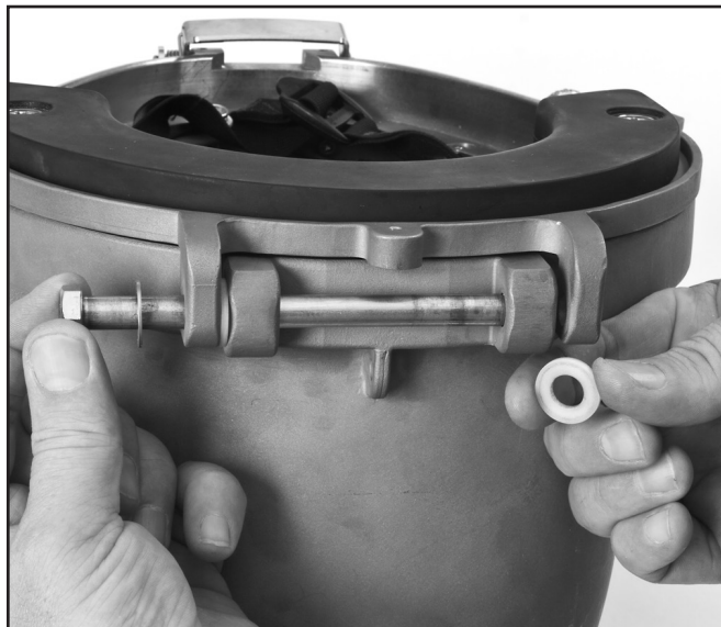
Make sure to re-install the Teflon® washers.
