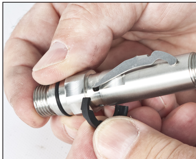
Remove the bearing clip.
