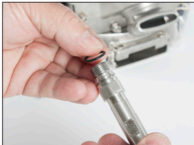
Remove the O-ring from the main tube.
