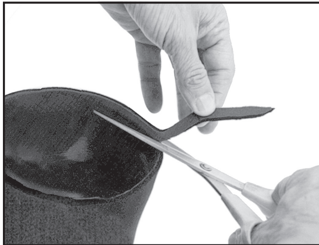
Trimming the neck dam.
