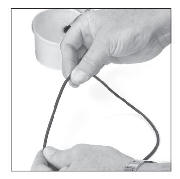
Lightly lubricate the port O-ring prior to installing it into the face port O-ring groove.
