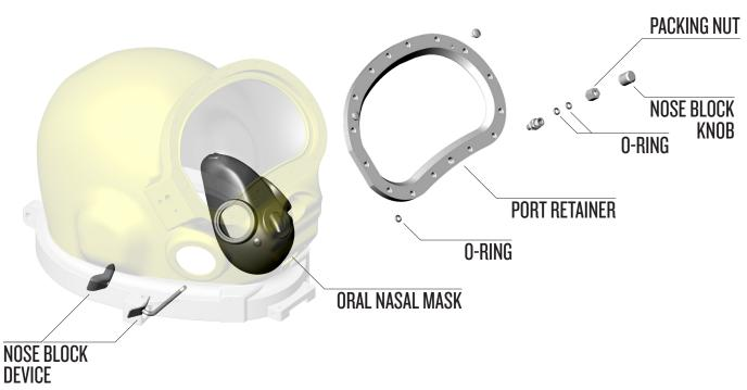
Blowapart of the nose block device and supporting hardware. (Same as found on KMB BandMasks).
