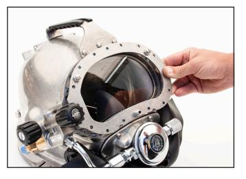
Place the port retainer on the helmet or mask shell.
