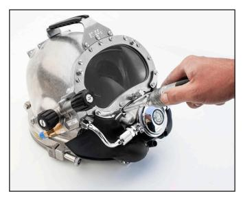
Remove the screws that secure the port retainer.
