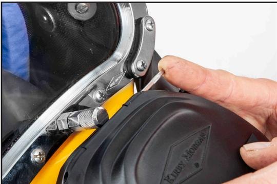
16) Align the access cover, P/N 510-733, to the regulator shroud P/N 510-723, as shown and install the pin, P/N 550-644, until it is evenly located into the area of the regulator shroud where it will remain.
