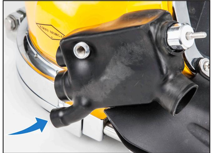
6) Reinstall all of the side block parts that were removed except the bent tube assembly.
