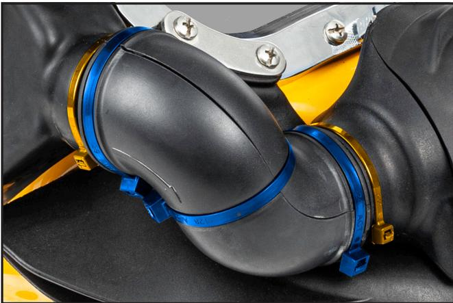
14) Secure the two tubes in this position using the wider tie wraps first.
