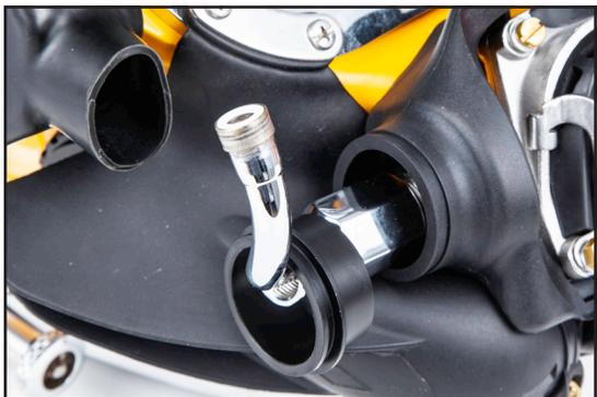
10) Swing the bent tube away from the side block and put the adapter sleeve (short, P/N 550-572), onto the bent tube assembly first, channeled end facing away from regulator inlet.
