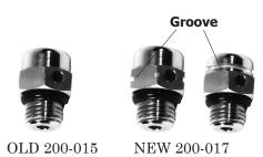
Do not use the older KMDSI Overpressure Valve Part # 200-015. It does not have the groove cut in the valve body.
