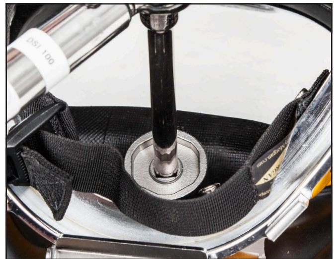
Removal of the regulator mount nut.
