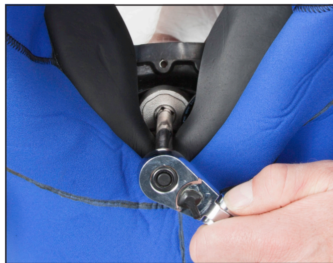
Removal of the regulator mount nut.
