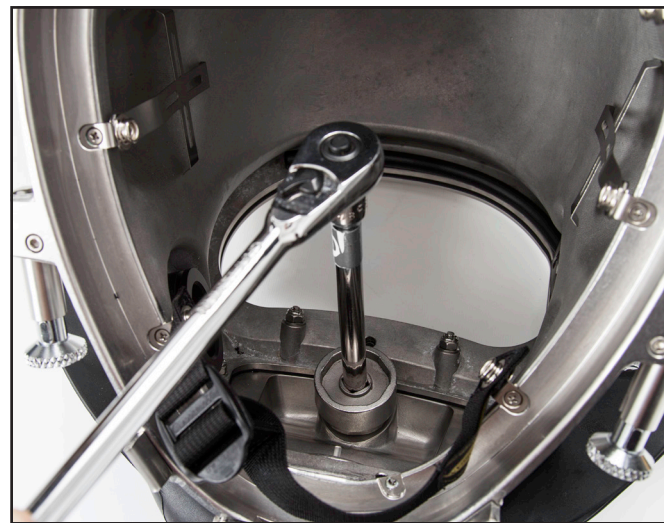
Removal of the regulator mount nut.
