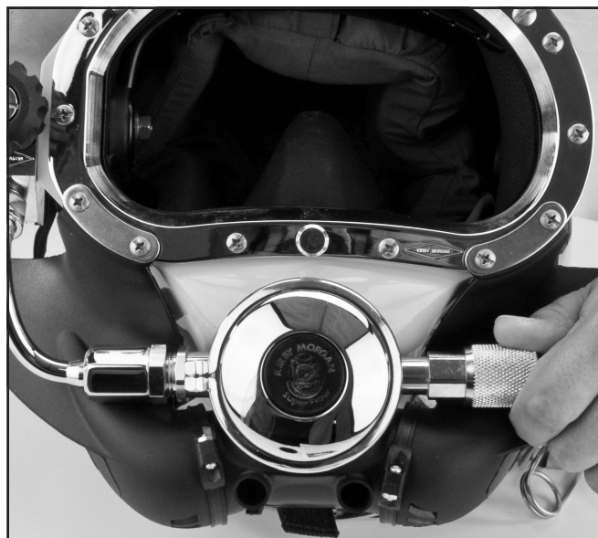
The regulator should begin to free flow once the adjustment knob is screwed out several turns.
