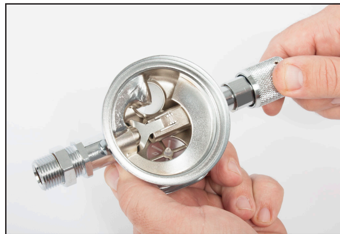
The adjustment assembly must turn freely.
