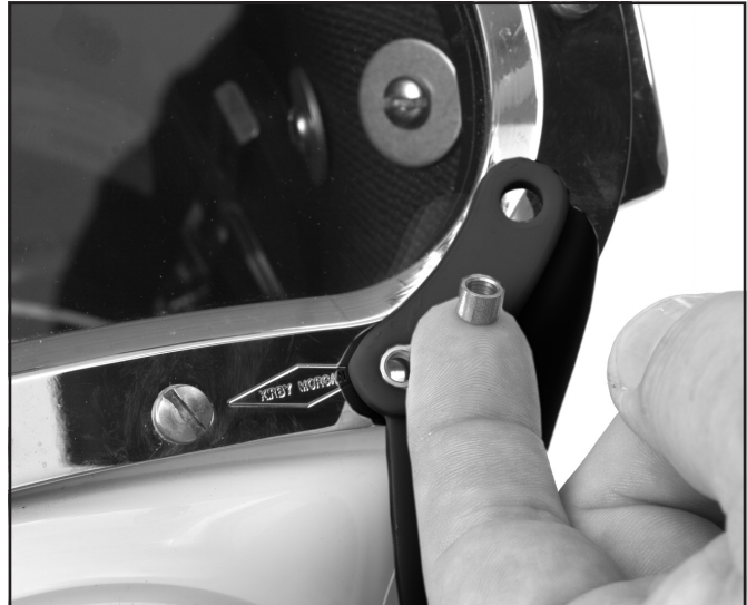
Make sure to replace the whisker spacers when you reinstall the whiskers.
