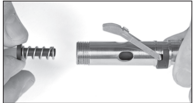
Insert the balance spacer and spring in the main tube. When it is properly installed the spacer will engage the inlet valve.
