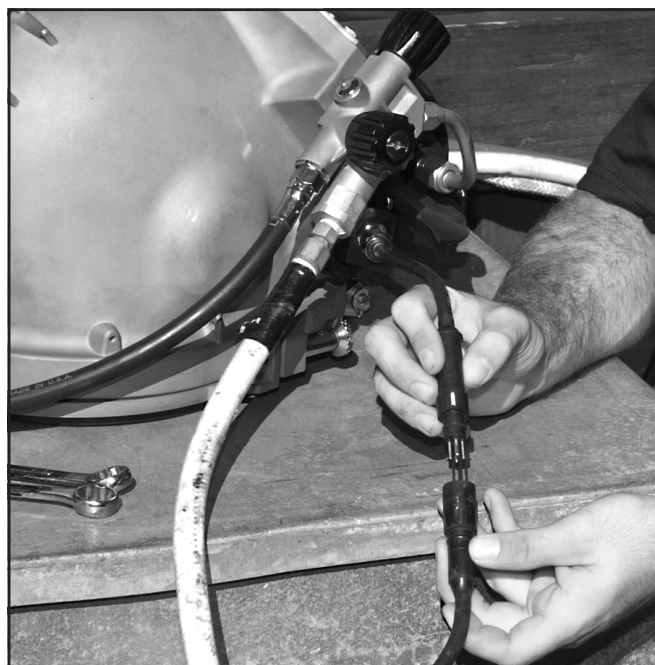
Connecting the waterproof connectors.
