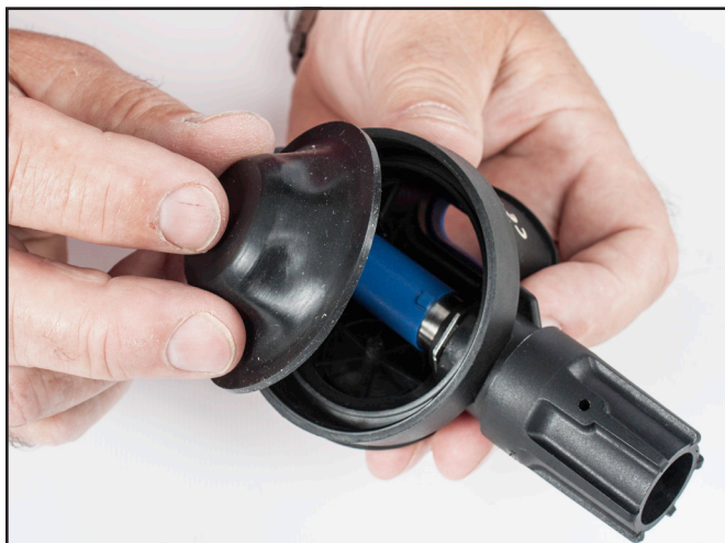
Install the diaphragm.
