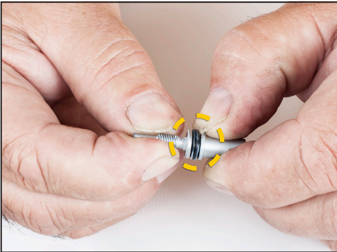
Remove the O-ring.
