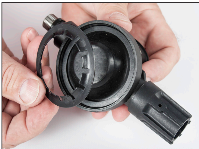
Install diaphragm surge dam.
