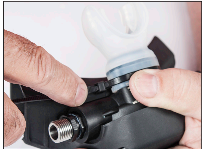
Install the tie wrap.
