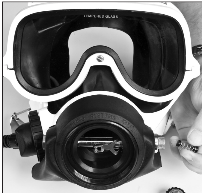
Installation of the spring set.
