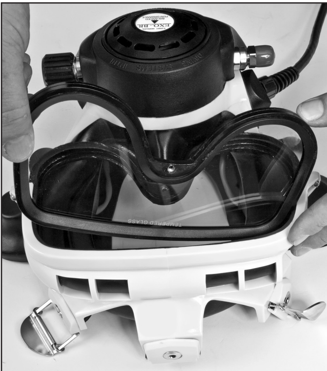
Install the right side of the lens rim into the channel of the rubber on the mask seal.
