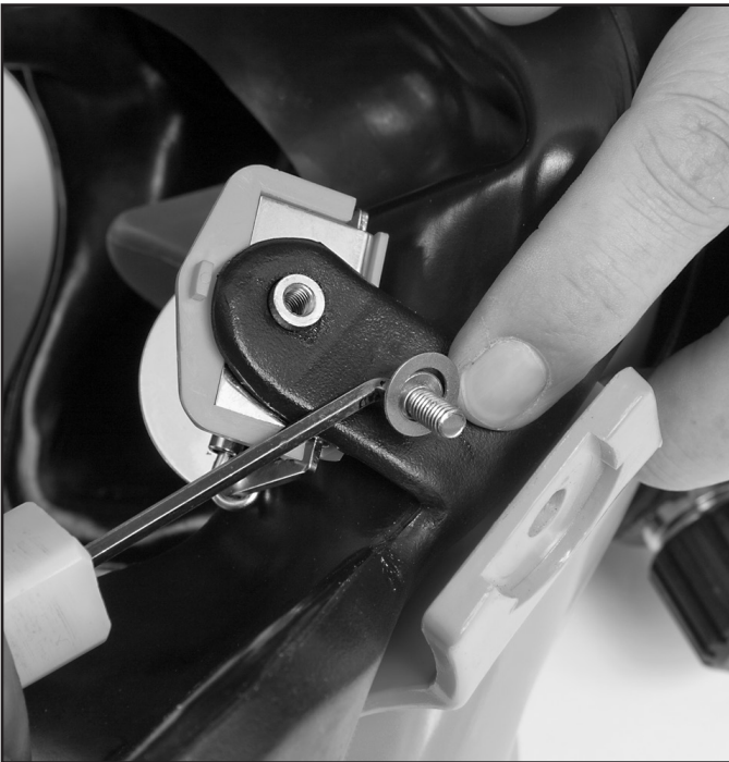
Insert the screw through the mask frame.
