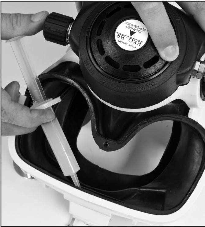
Apply silicone grease to the mask seal.
