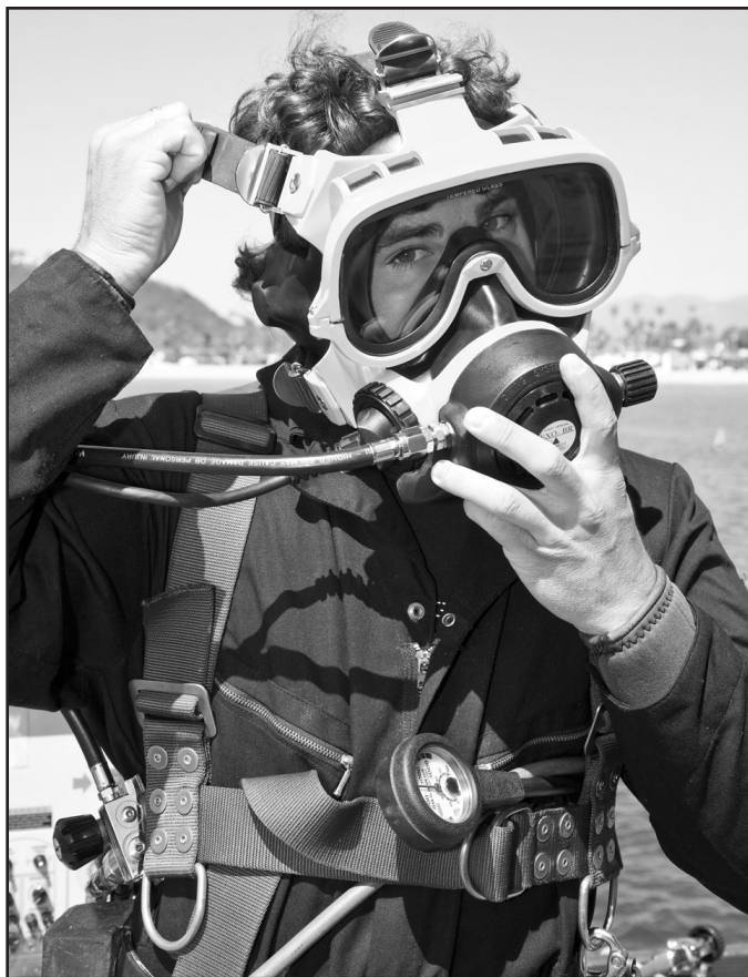
Tighten the upper spider legs next.
