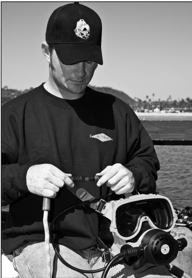
Connect the waterproof connectors without twisting them.
