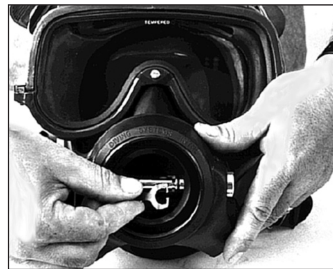
Remove the roller lever arm.
