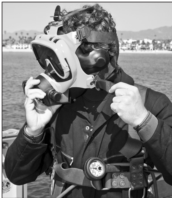
Tighten the lower spider legs first.
