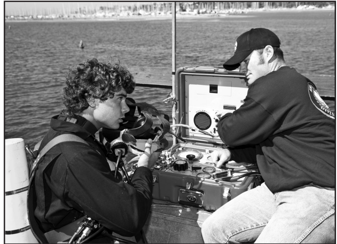
Always test the communications before the diver gets in the water.
