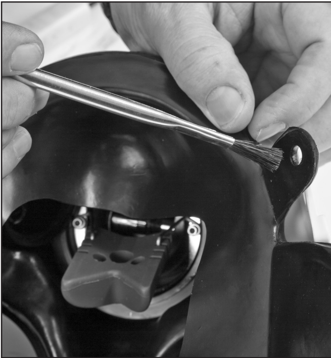
Lightly lubricate the screw hole on the spider tab.
