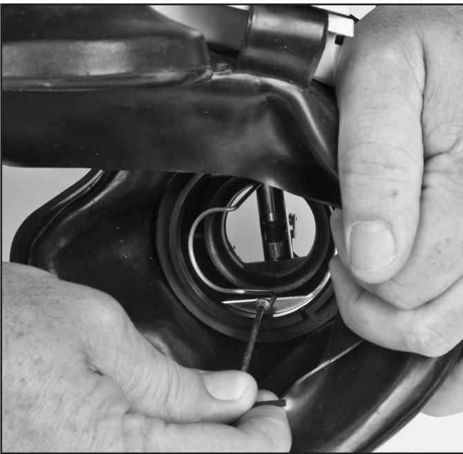
Tighten the screws for the nose block wire retainer.
