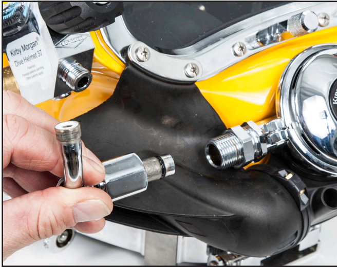
Removing the bent tube.
