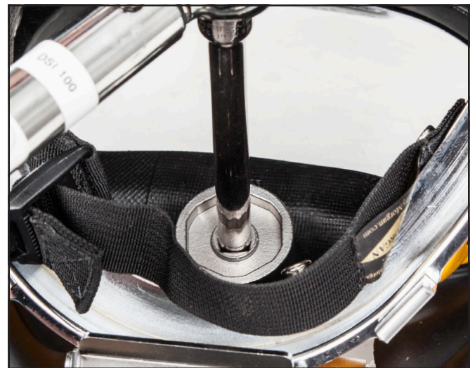
Removal of the regulator mount nut.
