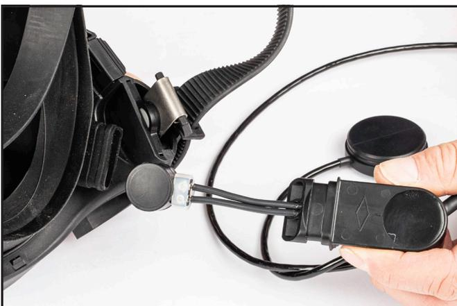
2) Push the microphone into the port. (The microphone will appear to be too large, but the seal easily stretches.)
