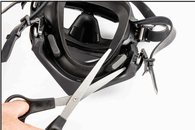
1) Using a sharp pair of scissors cut off the end of one of the communications ports, located below the bottom edge of the mask frame.
