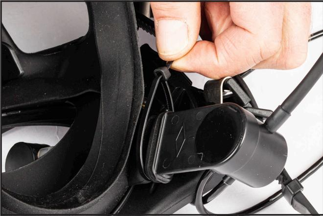
3) Use the included tie wrap P/N 520-038 to secure the communications assembly to the mask. Position the end or termination of the tie wrap so it won't be touching the diver's face.
