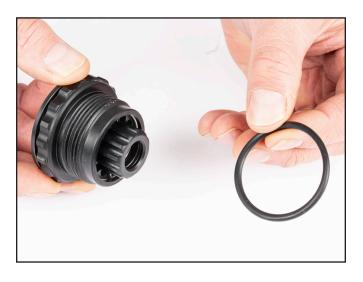
2) Use pick to remove Retaining Ring.
