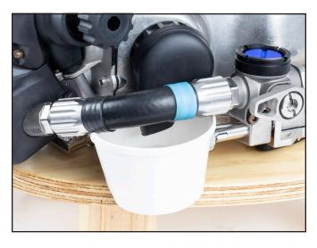
3) While maintaining a steady flow of gas through helmet, press and hold stem on exhaust assembly.
