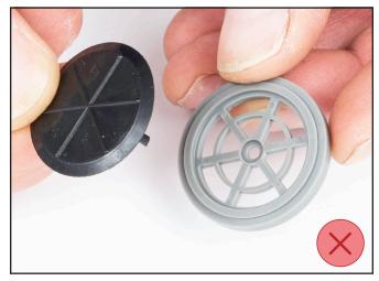
5) Insert Valve Insert with valve installed into main body.
