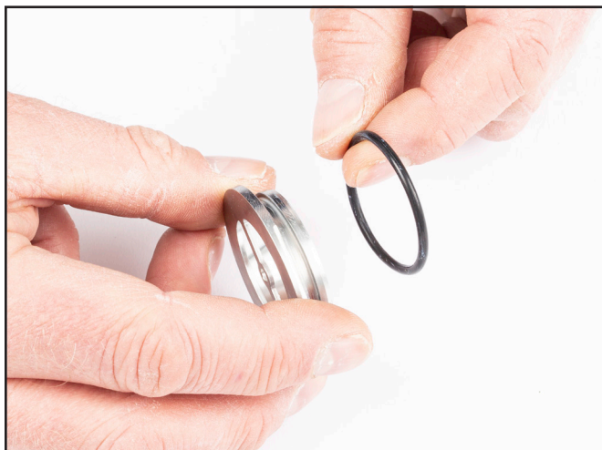
13) Remove Housing Retainer Ring.
