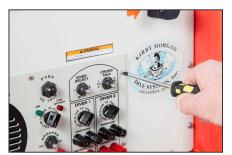
Remove the six screws using a #2 Phillips screwdriver and set aside in a safe place where they will not be lost.
