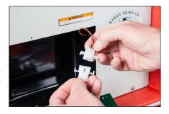
Disconnect the battery connectors by simply pulling them apart and complete separation is possible.
