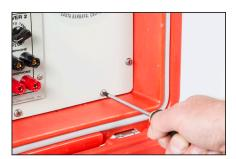
To replace the battery, remove the screws which hold the communicator panel into the top of the KMACS 5 box. Do not remove the screws which secure the communicator to the larger panel. Tilt the panel out but do not remove it from the lid.
