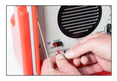
Match the Red and Black probes to the Red and Black receiving holes on the lower left panel of the communicator to connect the charge to the MK3-KMDSI communicator.
