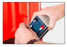
The battery is held in place by brackets and Velcro® strips on the back of the large panel. Reach behind the panel and support the battery. Lift the panel and battery out as a unit.
