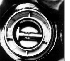
Incorrect, The lip of the mask seal on the lower right side has pushed through the frame.
