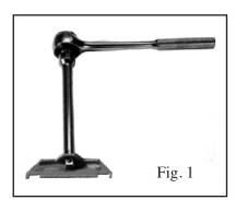
Put the regulator mount nut tool on the ratchet as shown.
