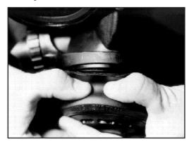
Incorrect, the whisker is not properly seated. The lip of the whisker seal has come out of the frame.
