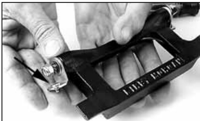
Install the screws through the mount ears.
