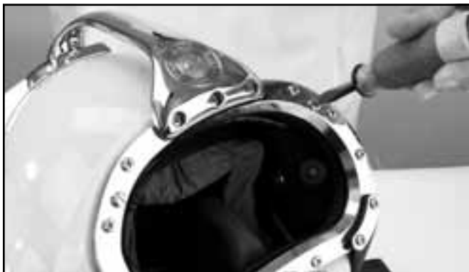
Remove the two plug screws from the port retainer.
