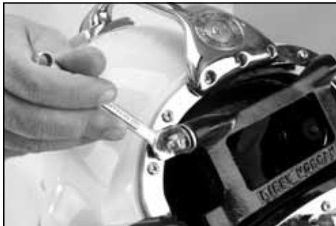
Tighten the weld lens assembly.
