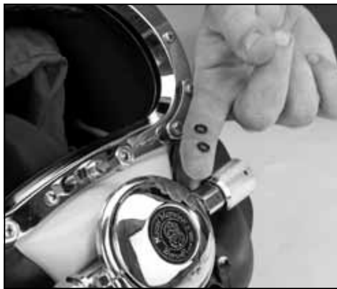
The nose block o-rings must be regularly lubricated.
