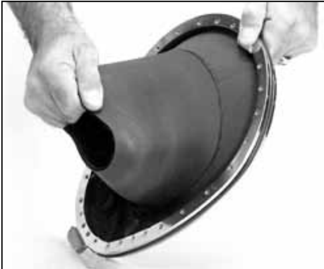
Check the neck dam for holes and compress between the rings.
