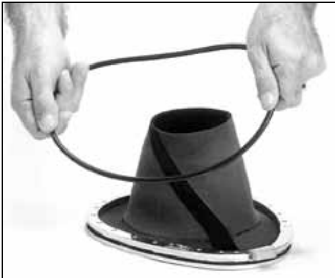
Inspect the o-ring on the neck dam ring.
