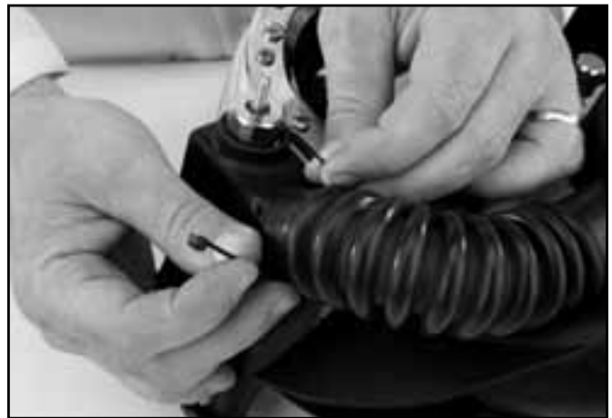
Install the corrugated tube and secure with tie-wraps.
