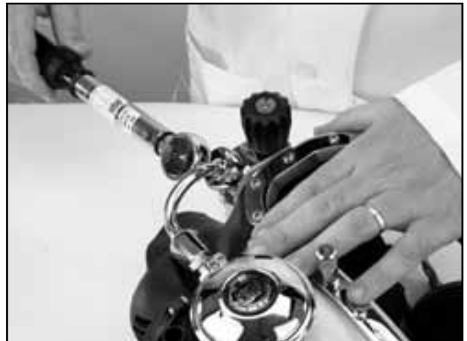
Loosen the bent tube.
