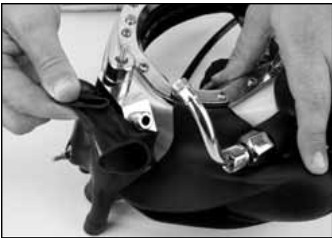
Position the shroud over the side block.
