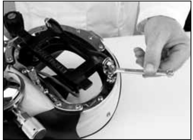
Tighten the weld lens assembly.
