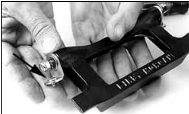
Install the screws through the mount ears.
