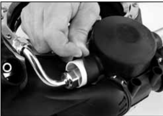
Slide one of the PVC pieces over the bent tube and insert it into the regulator shroud.
