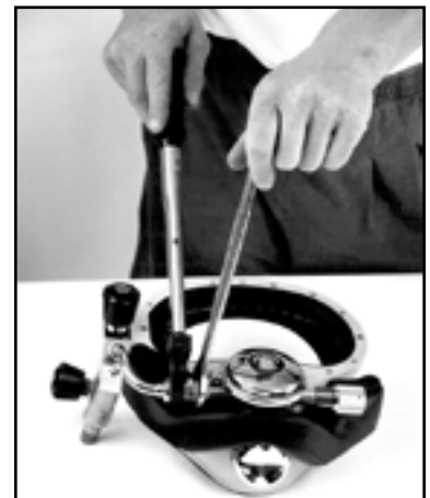
Tighten the Jam Nut using two wrenches
