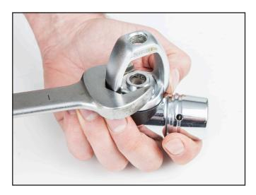
26) Thread the Yoke retainer, saddle and yoke as an assembly into the regulator body.
