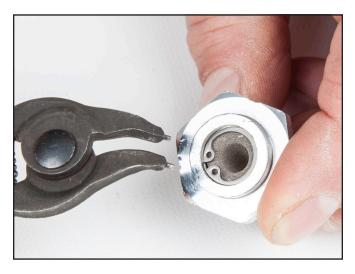
18) Remove and inspect the filter for oxidation and contamination. If the filter is corroded or shows visual signs of contamination it must be replaced. When in doubt, replace the filter.
