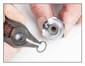
22) Install the two O-rings on the yoke retainer.
