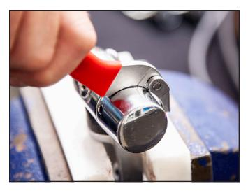
3) Remove the end cap from the regulator body. The piston/spring assembly will come away with
