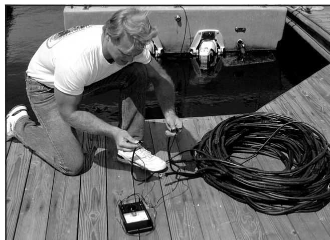
Preliminary testing of the umbilical with a volt-ohm meter to check for continuity.
