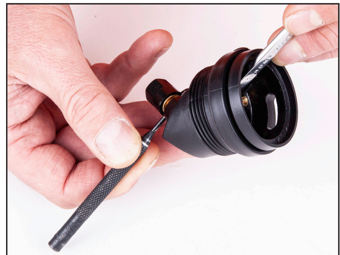
Use a wrench and \frac{3}{32} punch or small drill bit to tighten the communication post nuts.
