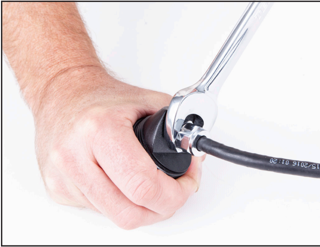
Use a 3/4 inch wrench to unscrew the waterproof connector.
