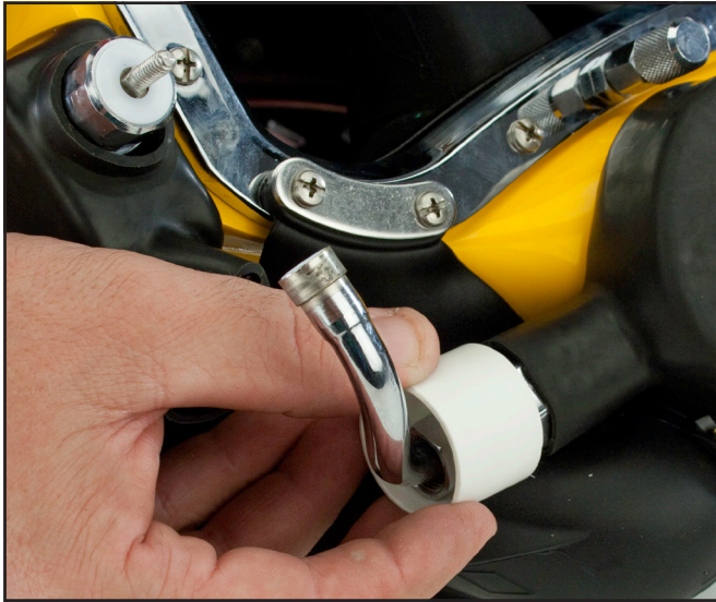
Slide one of the PVC pieces over the bent tube and insert it into the regulator shroud.
