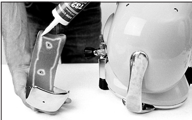
RTV (silicone sealant) is used to seal the weights to the helmet shell.
